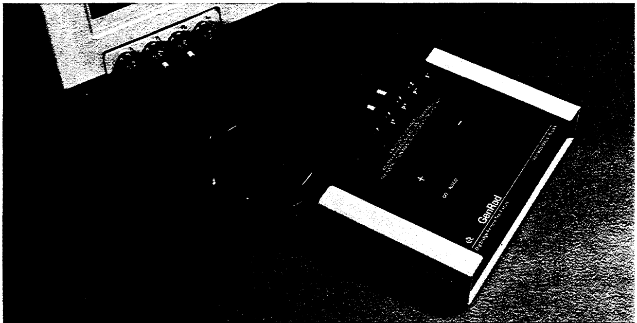
Figure 3-3. Remote test fixture (1689-9605), connected to a Digibridge tester.
